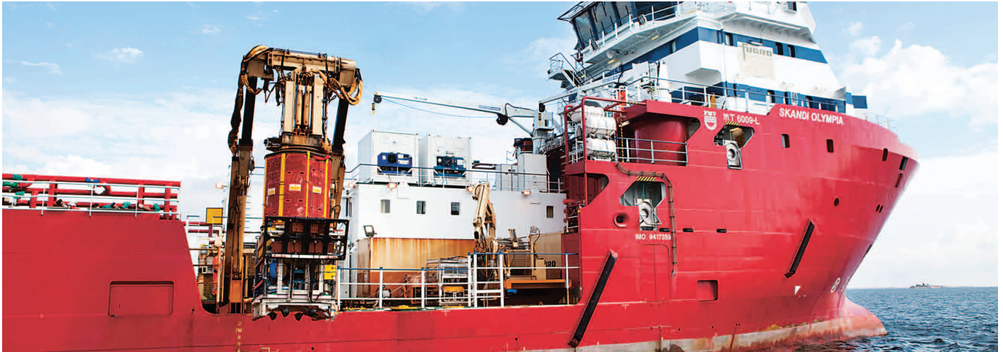
The survey vessel, Skandi Olympia is deploying a remotely operated vehicle that is used for visual inspection of the pipeline.
