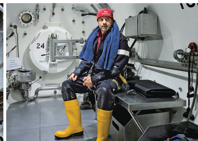
Technical divers, including Einar Flaa, live in special accommodations pressurised to match the pressure on the seafloor where they will work.
