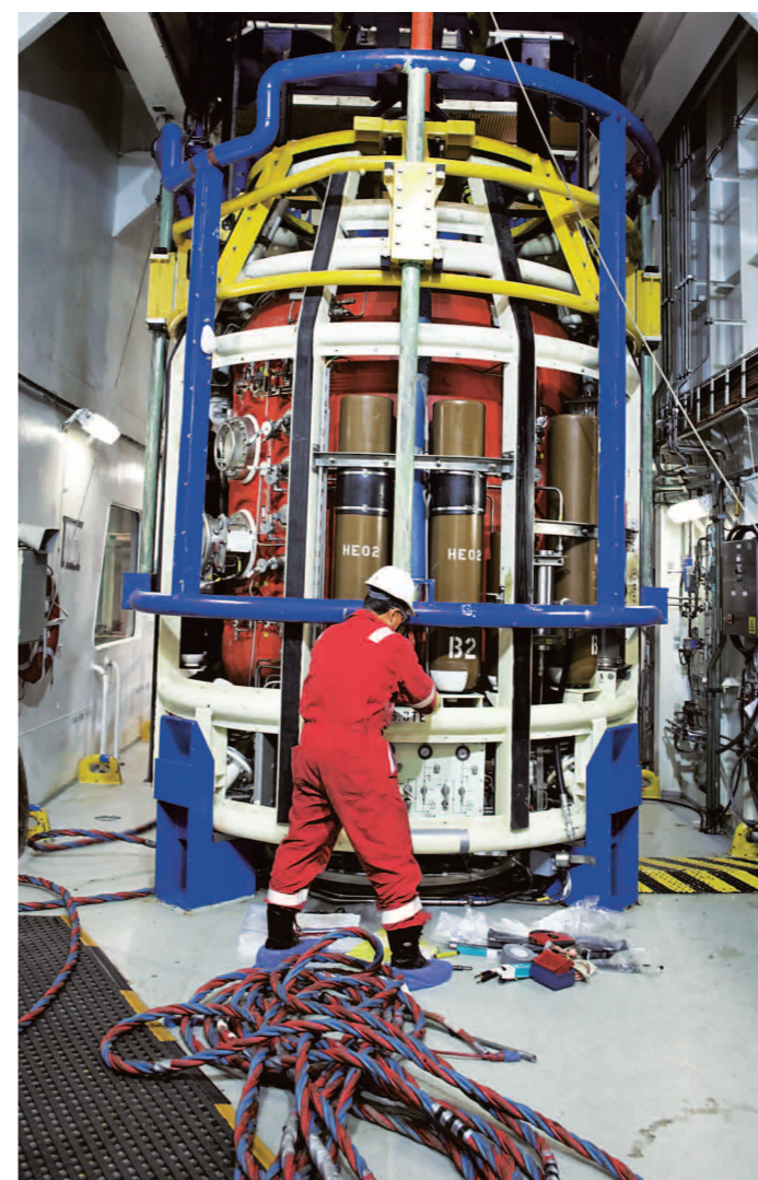
A three-man diving bell brings the divers from the pressurised diving system where they live to their subsea work area.
