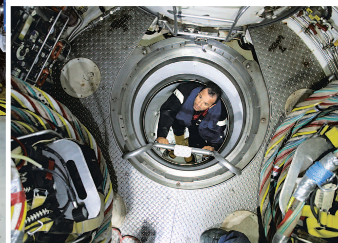
Flaa enters the diving bell from the diving system he lives in during the hyperbaric tie-in work for Nord Stream.
